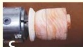
The bowl blank is attached with hot-melt adhesive. To achieve a strong bond, the tailstock was used for pressure during the curing process.
