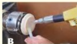
First apply a thin layer of hot melt adhesive to an auxiliary blank using a heat gun. Hot melt adhesive will also be applied to the rim of the bowl blank.
