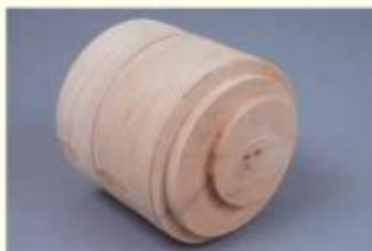
This roughed-out blank shows the offset tenons. (The recess in the other end is not shown.) After several months of drying, the blank is remounted and each tenon is trued. The balanced bowl is then made following the steps in the article.
