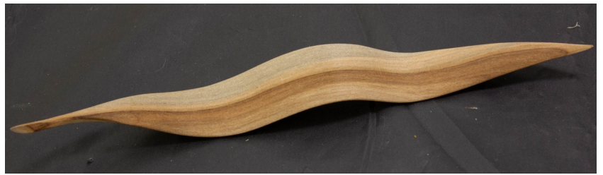
Bent compressed wood
