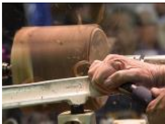
Roughing Cuts with Bowl Gouge
