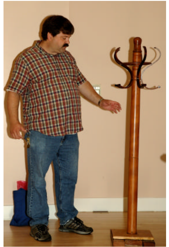
Chris Beck's turned coat rack. Chris added lead weight to base for good stability.
